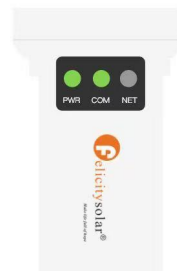
Normal communication with solar device
